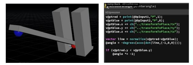
For the vertical movement, I use intersection analysis node to figure out where the intersection between the plank and the pole is. First, I deleted all the faces from the plank except for the one that first intersect with the pole and divide it in the middle vertically. Then, I used the intersection analysis to find the point of the intersection.
