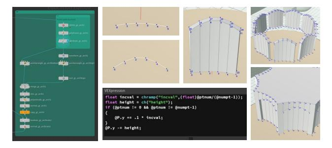
The initial curve is taken, and two of the endpoints are deleted. The above VEXpression is used to manipulate the Y-values based on a ramp. The curve manipulated into an arch and the initial curve with the culled endpoints are used to generate a surface through Polyskin, then extruded. This shape is rotated, and a Boolean Subtract node is used to cut into the initial building mass. VEXPression developed by Professor Deborah Fowler.
