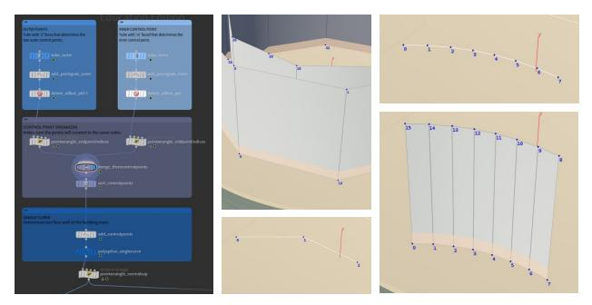
To create the one curved wall face for the radial building, two tubes were used, one for the midpoint and one for the endpoints. These were used to create the control points for a curve created by a Polyspline node. This curve was copied and a Polyskin node was used to create one wall. Solution developed by Professor Deborah Fowler.
